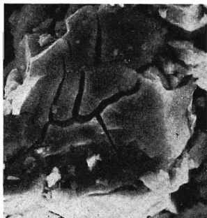
FIG. 11 Surface of Ni catalyst dried on the air at controlled temperature. Magnification 3 000 \times
