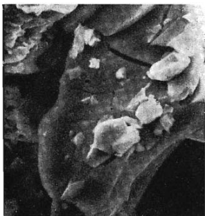
FIG. 10 Surface of Ni catalyst inactivated by hydrogen peroxide and dried on the air. Magnification 3000 \times
