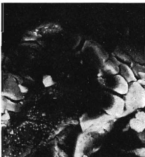
FIG. 12 Surface of Ni catalyst oxidised pyroforically by air. Magnification 3 000 \times
